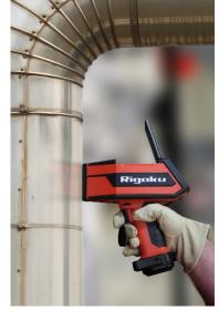
steels, stainless steels, as well as high temperature alloys and the added detection of lithium (Li). In addition, the KT-100S analyzer offers unique auto surface preparation with its Drill-Down™ feature and is considerably smaller and lighter than other handheld LIBS analyzers currently available.
